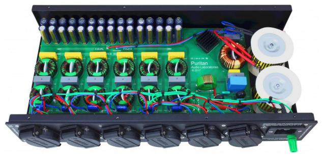
Designer and Puritan boss, Mike Lester commented, "So the PSM156 aim was to eliminate the need for overcurrent protection in the box with the fuse in the plug of the power lead providing the overall safety (Schuko, Nema, etc. versions have a single internal 15A fuse as these plugs
